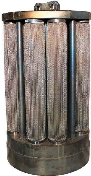
Filter bundle after plastic removal
