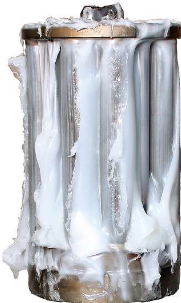
Filter bundle before plastic removal
