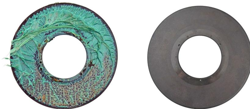
Laser filters can be quickly and safely freed of plastic residues with the aid of thermal vacuum pyrolysis. Here before and after cleaning in a VACUCLEAN system
