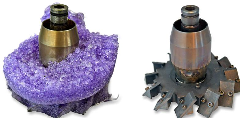
The use of thermal cleaning to remove plastics from machine parts, such as pelletizer knives, significantly increases machine availability, reduces costs and increases productivity. Here before and after cleaning in a VACUCLEAN system
