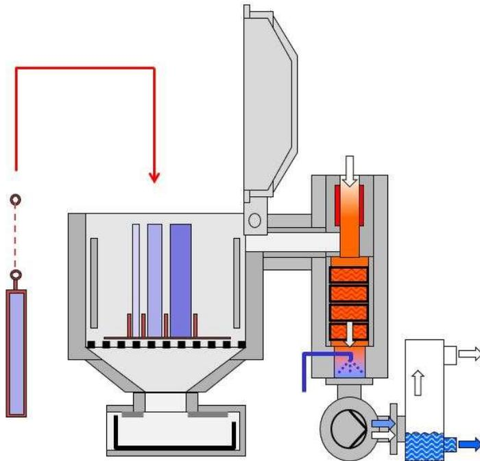
Functional principle of thermal vacuum pyrolysis: The cleaning process takes place in an electrically heated vacuum cleaning chamber. The temperature is measured directly at the machine parts, which are initially heated slowly and particularly gently. Here, a large part of the adhering polymer melts off and flows out. The decomposition of the remaining material takes place at approx. 450 degrees Celsius - remaining carbon is finally removed by adding air (oxidation)
