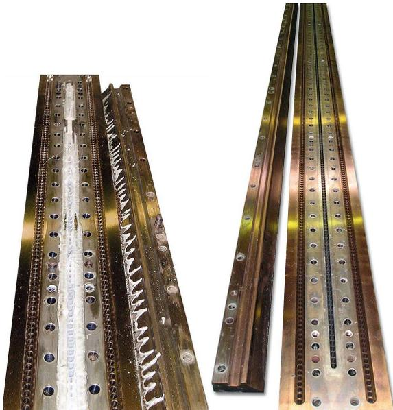
Melt-blown dies before and after cleaning: An optimized cleaning process with thermal pyrolysis, two side sound and further post-treatment removes polymer residues from machine parts in the nonwovens industry
