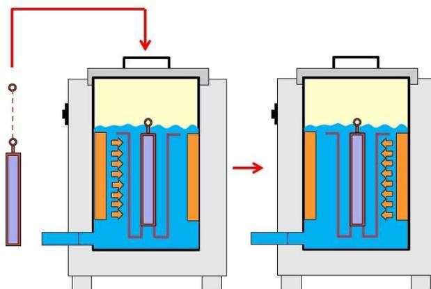
Functional principle of the optimized cleaning process with switchable two-side sound: Thanks to switchable two-side sound, machine parts no longer have to be rotated
