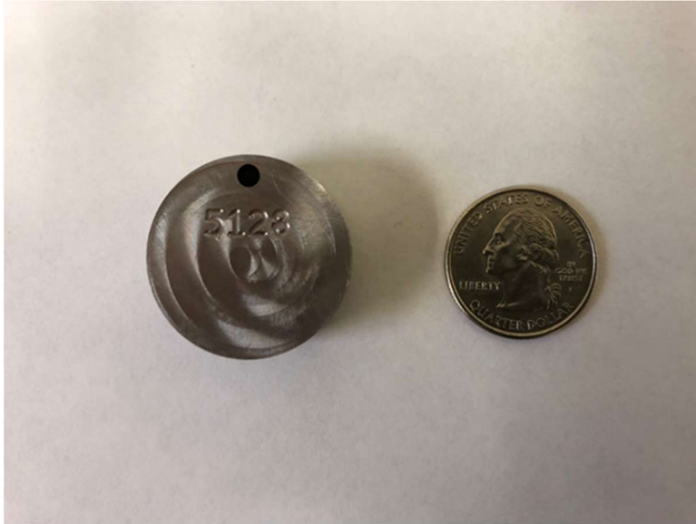
Figure 3: Typical sample used for the austempering trials compared to a US quarter Dollar coin Photo credit: SCHWING Technologies Download: https://drive.google.com/file/d/1WK-zY9WYVW-vAyjiw0Zu4a37P7edq_UB/view?usp=sharing
